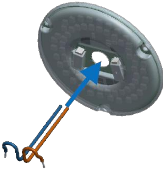
1 Insert the AC wire into the cover hole. When you m
