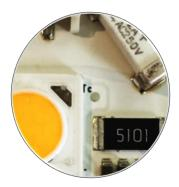
The lifetime is calculated at the maximum temperature recommended at the Tc (measuring point). It is important not to exceed this recommendation.
