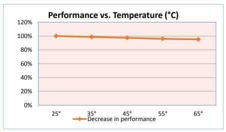
Consider the thermal capabilities of where the LED module is to be fitted. The temperature is an important factor for light output as well as for long time light output degradation.
