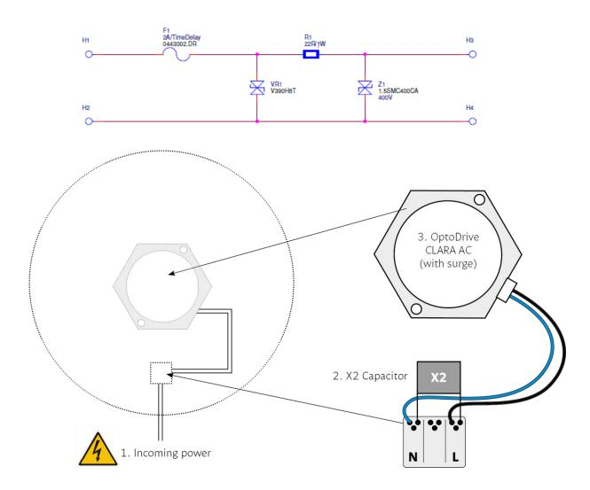
The installation set up requires an X2 Capacitor parallel to L1 and N to handle the fast and high voltage transients generated by the magnetic ballast.
