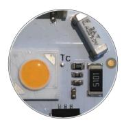
The lifetime is calculated at the maximum temperature recommended at the Tc (measuring point). It is important not to exceed this recommendation.
